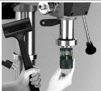
4. Mounting/removing drills / morse taper:
